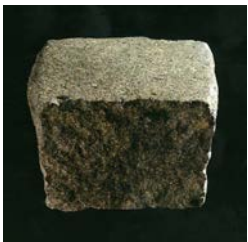
Fig. 4 Roads: Porphyry cobblestones or sandstone, rectangular shape
