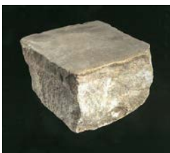
Fig. 4 Roads: Porphyry cobblestones or sandstone, rectangular shape
